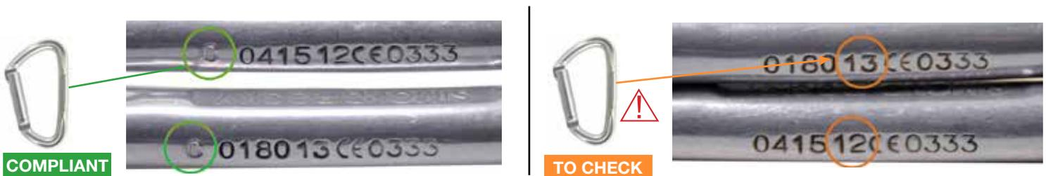
Photo n°3: serial numbers with the year of manufacture already passed and those to be checked
